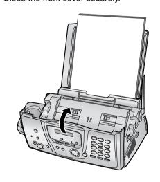
**8** Remove the recording paper and straighten. Pull the tension plate forward (①) and insert the paper. Then push the tension plate back.
